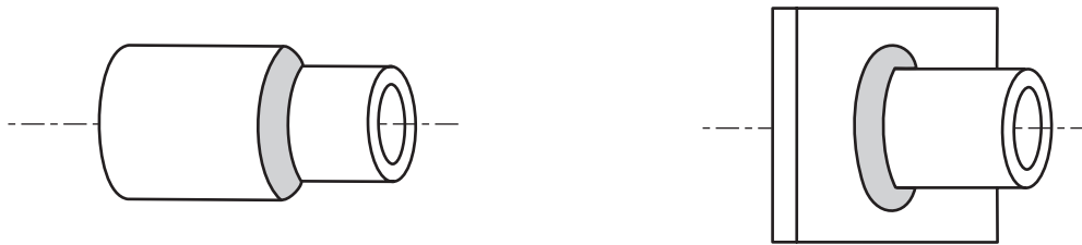
(E) MULTIPLE WELDING TEST POSITION—5F
