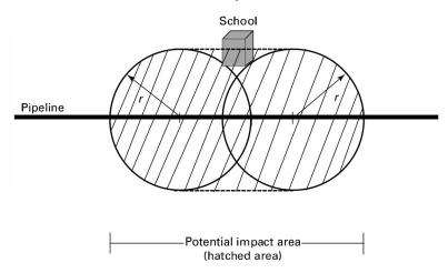
GENERAL NOTE: This diagram represents the results for a 30 in. (762 mm) pipe with an MAOP of 1,000 psig (6900 kPa).
