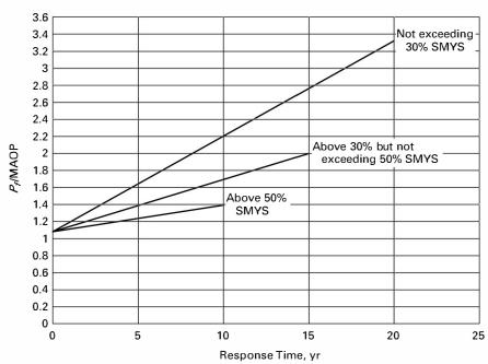
GENERAL NOTE: Predicted failure pressure,  $P_{f_0}$  is calculated using a proven engineering method for evaluating the remaining strength of corroded pipe. The failure pressure ratio is used to categorize a defect as immediate, scheduled, or monitored.
