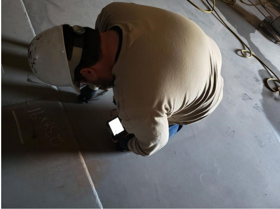
Figure A.3—Ultrasonic Examination
