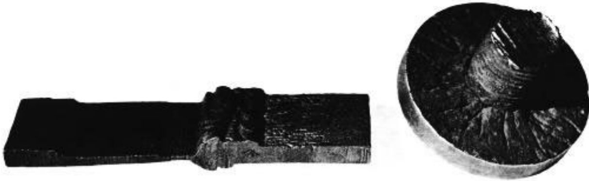
Figure 26—Caustic Stress Corrosion Cracks
