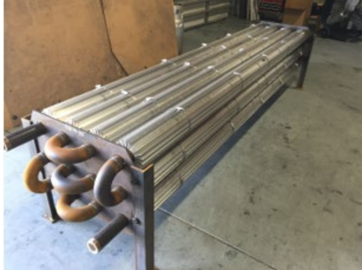
Figure 43—Fin-tube Type of Heaters Commonly Used in Storage Tanks
