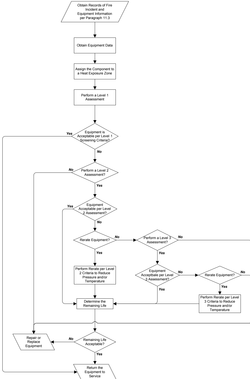
Figure 11.1 Overview of the Procedure to Evaluate a Component with Fire Damage
