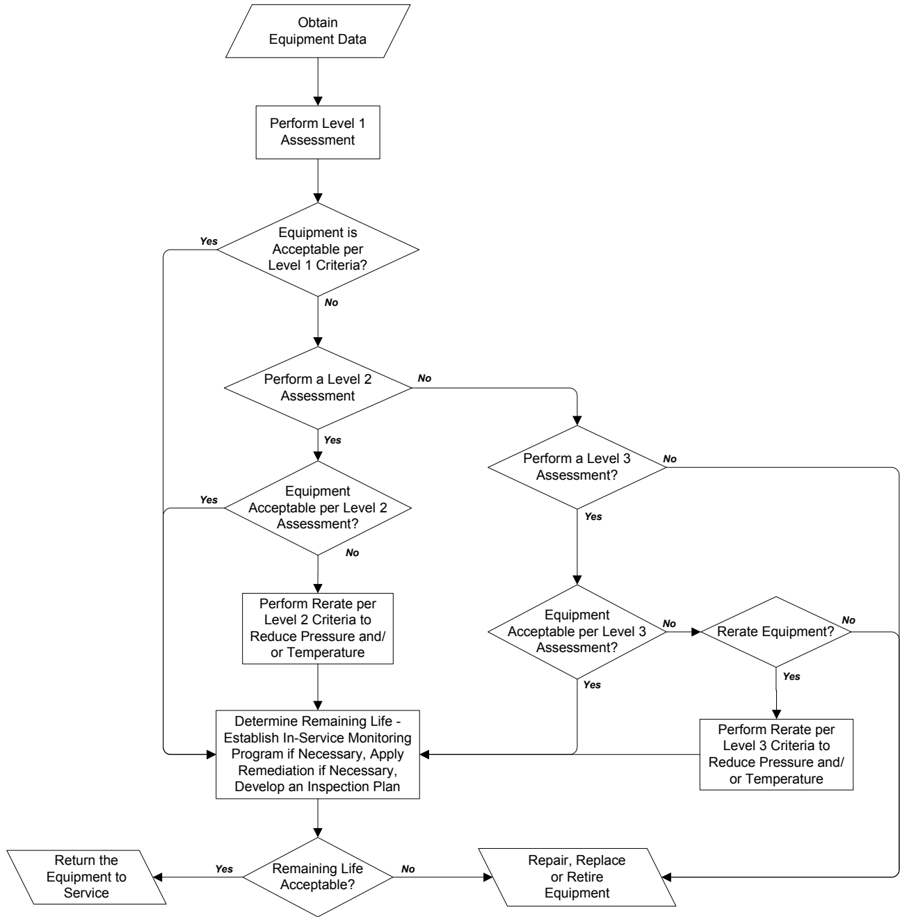
Figure 7.1 – Overview of the Assessment Procedure to Evaluate a Component with HIC or Hydrogen Blisters
