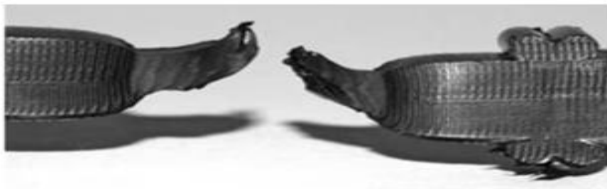
Ductile Rupture Outside Fusion Interface
